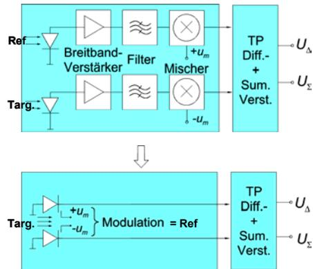
Fig. 2. Comparison of a) the conventional and b) the new PMD-receiver concept of LED/Laser-Ranging by echo TOF (shown without optical sender)
