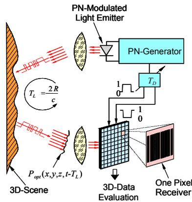
Fig. 1. In this PMD-camera each PMD-receiver operates as a 1D-laser radar but here in a PMD-matrix in parallel and at the same time.
