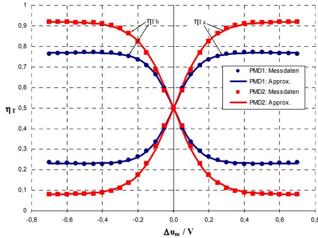
Fig. 4. Modulation characteristic describing the photo current distribution over the odd-mode modulation voltage  $\Delta u_m$  [8]
