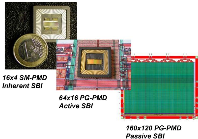
Fig. 9. Three PMD-matrices: a) 64 SM-MSM / OEP-PMD-pixels, b) 1024 Photo-Gate PMD-pixels and c) Layout of a 19200 Photo-Gate PMD-pixel array.
