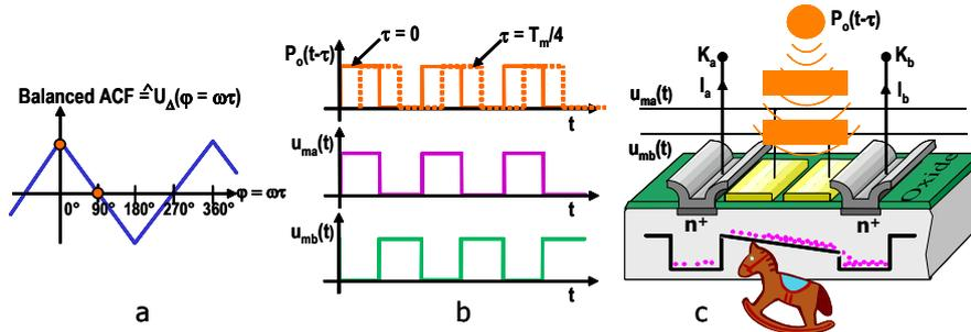
Fig. 3. c) PMD operates like a voltage seesaw for photo electrons generated below the balanced modulated photo-gates thus mixing by anti-symmetrical sampling to the left and to the right. b) At a light-wave phase zero the total charge drifts to the positive right side with maximum charge difference; at  $90^\circ$ : equally distributed charge results in zero difference. a) The charge or voltage difference described by the balanced Auto-Correlation-Function is a measure for delay.
