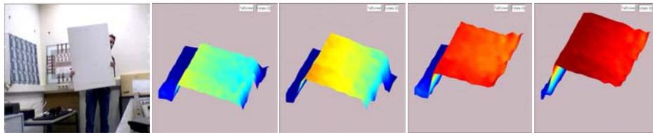
Fig. 6. Four 3D-snapshots out of a 50Hz video sequence show the upwards moving pale board in color coded height
