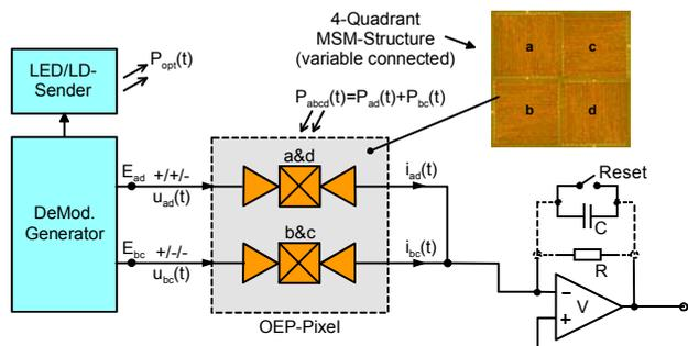
Fig. 3. 4-Quadrant multi-functional MSM-OEP-pixel for OE-logic, 3D-sampling, routing, etc.
