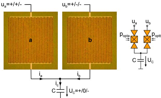
Fig. 1. Basic OEP-structure formed by two MSM-PMDs, being switched off at odd polarity
