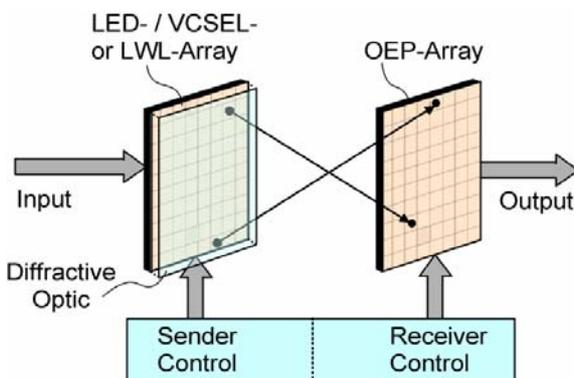
Fig.5. Scheme of an optical PMD / OEP-cross connect and router
