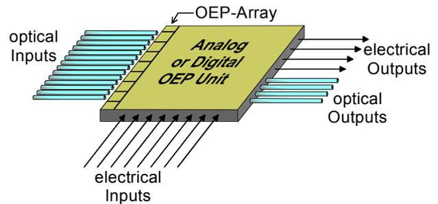
Fig.6. A general, programmable OEP-Unit for multi-channel analog and digital OE-signal processing
