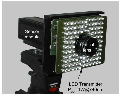
**Figure 6: 3D camera module on tripod**
